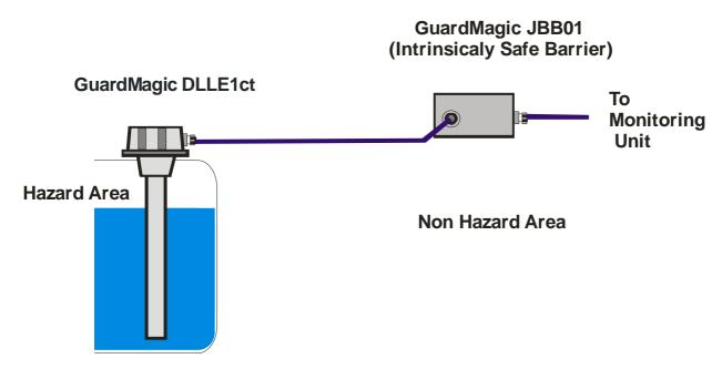
GuardMagic DLLE1 fuel level sensor working only together with GuardMagic JBB01 Intrinsicaly Safe barrier.
